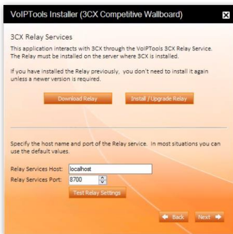
Figure 2: Test VoIPTools 3CX Relay settings
